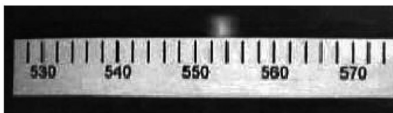
FIGURE 6 Lasing spectrum of a pyrromethene dye (No 567) in NLC Zhk-654.
